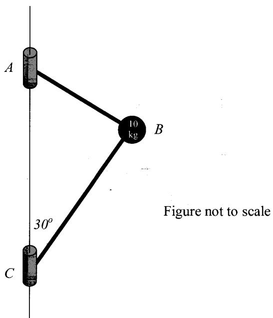
The above diagram shows a mass of 10 kilograms at  $B$  connected by light rods (at right angles) to sleeves  $A$  and  $C$  which revolve freely about the vertical axis  $AC$  but do not move vertically. The angle between the vertical axis  $AC$  and the light rod  $BC$  is  $30^\circ$ . The acceleration due to gravity is  $g$  metres per second squared.
